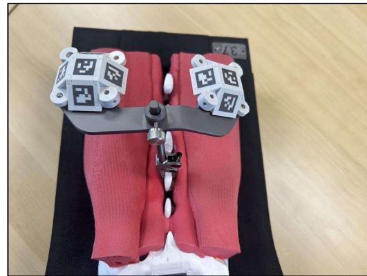
Figure 1 Spine Clamp (S-S) with small patient trackers
